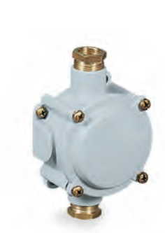
NAVE SERIES Watertight UNAV 1398 junction box in brass painted marine grey, with terminal block and UNAV 1948 cable glands IP66
