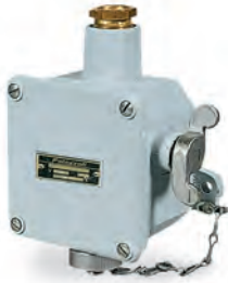
NAVE SERIES Watertight UNAV 1436 interlocked plugs in brass enclosure painted marine grey, with cable glands UNAV 1948 IP56
