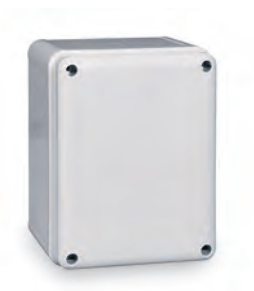
CAM-ST series Blind wall-mounted enclosure suitable for fitting a maximum of 2 rear panel devices screw or hole fixing IP65
