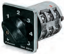
CAM SERIES 5-way + 0 watertight high performance selector switch with knob, front-plate and front panel Front panel IP65 Terminal blocks IP00
