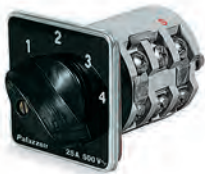
CAM SERIES 4-way + 0 watertight high performance selector switch with knob, front-plate and front panel Front panel IP65 Terminal blocks IP00
