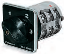
CAM SERIES 3-way + 0 watertight high performance selector switch with knob, front-plate and front panel Front panel IP65 Terminal blocks IP00
