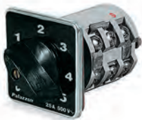
CAM SERIES 6-way watertight high performance selector switch with knob, front-plate and front panel Front panel IP65 Terminal blocks IP00
