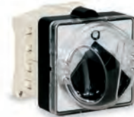
CAM-SZ Series Rear panel isolator switches with black knob and grey plate . Rear panel finish 67x67 IP65
